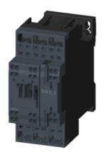
power contactor, AC-3 25 A, 11 kW / 400 V 1 NO + 1 NC, 230 V AC, 50 / 60 Hz, 3-pole, Size S0, Spring-type terminal upright mounting position
