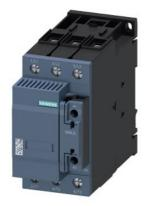
Capacitor contactor, AC-6b 50 kVAr, / 400 V 2 NC, 50-60 Hz AC / 20-33 V DC 3-pole, Size S2 screw terminal
