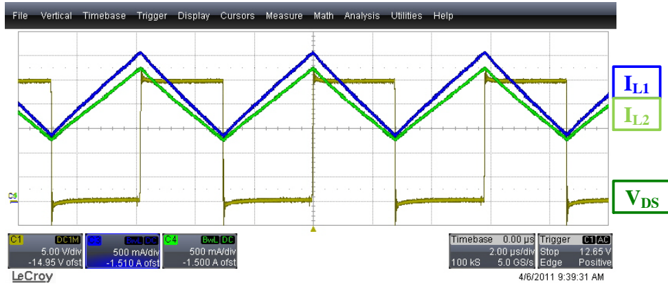
Figure 4. Operational Waveforms, V_{IN} = 12\text{ V} , R_{OUT} = 6\ \Omega
