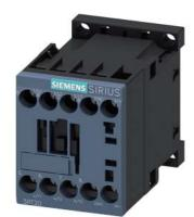
power contactor, AC-3 7 A, 3 kW / 400 V 1 NC, 24 V DC 0.85-1.85\* US, with diode integrated, 3-pole, size S00, screw terminal not expandable with auxiliary switch
