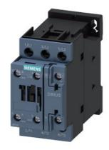
Power contactor, AC-3 38 A, 18.5 kW / 400 V 1 NO + 1 NC, 220 V AC 50/60 Hz, 3-pole Size S0, screw terminals
