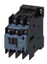
Traction contactor, AC-3 25 A, 11 kW / 400 V 1 NO + 1 NC with electronic drive 24 V DC, 0.7-1.25\* US, with integrated varistor, 3-pole, Size S0, ring cable lug connection
