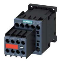
contactor relay, 4 NO + 4 NC, 110 V DC, size S00, screw terminal, captive auxiliary switch
