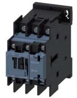
Power contactor, AC-3 38 A, 18.5 kW / 400 V 1 NO + 1 NC, 460 V AC 60Hz, 3-pole, size S0 ring cable lug connection
