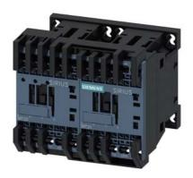
Reversing contactor assembly for 3RA27 AC3:  $5.5 \, kW/400 \, V$ ,  $24 \, V \, DC$  3-pole, Size S00 Spring-type terminal electrical and mechanical interlock with voltage tap
