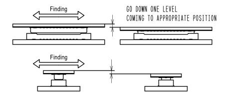
(2) WHEN GUIDING. THE CONNECTORS ARE ALIGNED PARALLEL TO EACH OTHER, WITH LONGITUDINAL AND LATERAL MOVEMENTS RESTRICTED. MATE THEM PROPERLY BY APPLYING FORCE IN THIS CONDITION.
