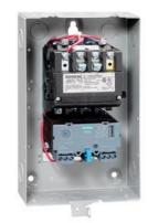
Non-reversing motor starter, Size 1, Three phase full voltage, Solid-state overload relay, OLR amp range 10-40A, Non-combination type, Enclosure type 1, Indoor general purpose use, Extra-wide enclosure
