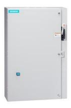
Non-reversing motor starter, Size 2 1/2, Three phase full voltage, Solidstate overload relay, OLR amp range 25-100A, 24VAC 50-60Hz coil, Combination type, 100A fusible disconnect, 100A/250V fuse clip, Enclosure NEMA type 1, Indoor general purpose use, Extra-wide enclosure
