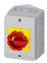
SENTRON, Switch disconnector 3LD, emergency switching-off switch, 3pole, Iu: 32 A, operating power / at AC-23 A 400 V: 11.5 kW, molded-plastic encapsulation for inch screw connection 4 NO, rotary operating mechanism, red/yellow
