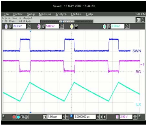
Figure 22. Switcher Operation – CCM Mode
