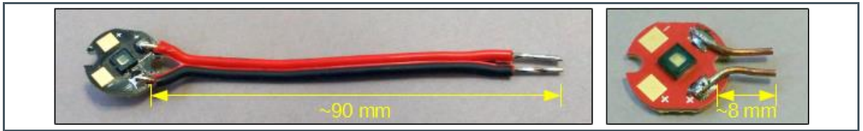
Figure 21: TARA2000-AUT / EGA2000 VCSEL Modules Mounted on Starboards with Different Wiring
