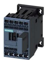
power contactor, AC-3 12 A, 5.5 kW / 400 V 1 NO, 24 V DC 0.85-1.85\* US, with varistor plugged on, 3-pole size S00, spring-type terminal not expandable with auxiliary switch
