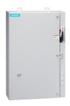
Non-reversing motor starter, Size 1, Three phase full voltage, Solid-state overload relay, OLR amp range 5.5-22A, Combination type, 25A circuit breaker, Encl NEMA type 4X 304 S-Steel, Water/dust tight noncorrosive, Extra-wide enclosure
