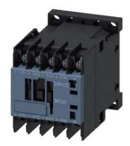
Power contactor, AC-3 9 A, 4 kW / 400 V 1 NC, 220 V AC, 50 Hz, 240 V 60 Hz, 3-pole, Size S00 ring cable lug connection
