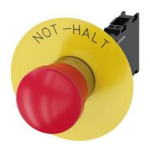
EMERGENCY STOP mushroom-type actuator, 22 mm, round, metal, shiny, red, 40 mm, positive latching, according to EN ISO 13850, pull-to-unlatch mechanism, with yellow backing plate, inscription: NOT-HALT, with holder, 1 NO+1 NC, spring-type terminal, Z=20-unit packaging
