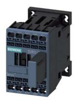
power contactor, AC-3 9 A, 4 kW / 400 V 1 NC, 24 V DC 0.7-1.25\* US, with varistor plugged on, 3-pole, size S00, spring-type terminal not expandable with auxiliary switch
