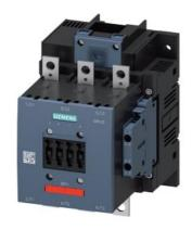
power contactor, AC-3 150 A, 75 kW / 400 V AC (50-60 Hz) / DC operation 23-26 V AC/DC auxiliary contacts 2 NO + 2 NC lateral, permanently mounted 3-pole, frame size S6 busbar connections
