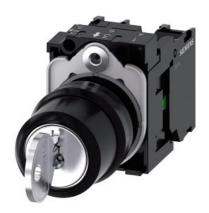
RONIS key-operated switch, 22 mm, round, plastic, lock number SB30, with 2 keys, 3 switch positions I-O-II, latching, 10:30h/12h/13:30h, Key removal I+O+II, with holder, 1 NO, 1 NO, screw terminal, possible special locks: SB31, 421, 455, with laser labeling, upper case
