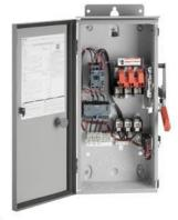
Slim Line Pump Control Panel NEMA size 1 Three phase full voltage Solid-state overload relay OLR amp range 0.75-3.4A 460VAC 60Hz Coil 30A fusible disconnect 30A/600V fuse clip 1NC / 1NO auxiliary contacts HOA Sel. Sw. <(>&<)> Start/Stop 3-point power terminal block 3-point control terminal block 3-point ground lug Enclosure NEMA type 3/3R Weather proof outdoor use
