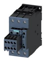
Contactor relay, AC-3 80 A, 37 kW / 400 V 2 NO + 2 NC, 24 V DC with varistor 3-pole, size S2 screw terminals suitable for 2 A PLC outputs
