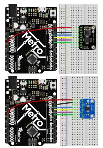
Connect Vcc to the power supply, 3V or 5V is fine. Use the same voltage that the microcontroller logic is based off of. For most Arduinos, that is 5V
