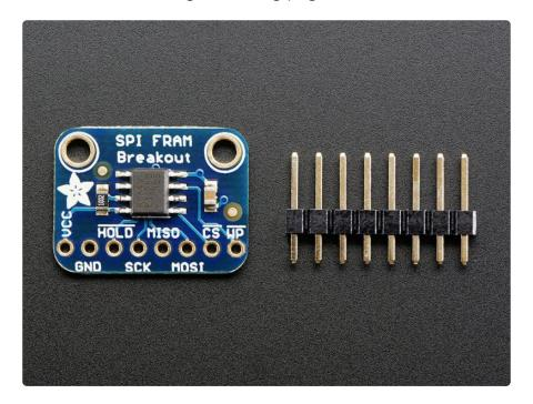
This particular FRAM chip has 64 Kbits (8 KBytes) of storage, interfaces using SPI, and can run at up to 20MHz SPI rates. Each byte can be read and written instantaneously (like SRAM) but will keep the memory for 95 years at room temperature. Each byte
