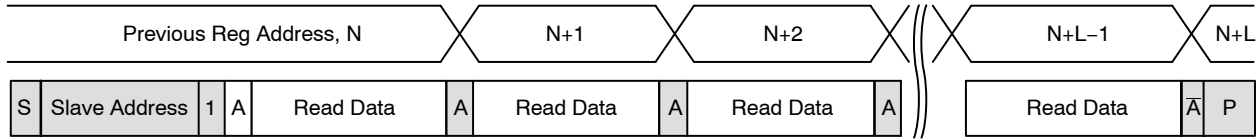
Figure 21. Sequential READ, Start from Current Location
