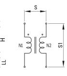
General InformationSeriesSC-GJStyleThrough-HoleRoHSYesNotesLead Spacing (S/S1) Are For Reference Only.MiscellaneousTemperature Rise Maximum: 40 K.CoreMn-Zn Ferrite
