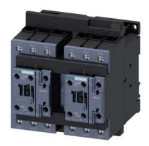
Reversing contactor assembly, AC-3, 30 kW 400 V, 220 V AC/50 Hz/240 V AC/60 Hz 3-pole, Size S2 screw terminal electrical and mechanical interlock 2 NO integrated
