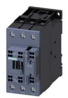
Power contactor, AC-3 80 A, 37 kW / 400 V 1 NO + 1 NC, 220 V AC, 50 Hz 240 V, 60Hz, 3-pole, Size S2, Spring-type terminals
