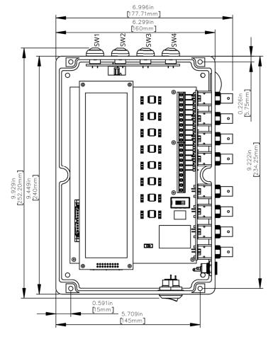
Use the following hole pattern if using the mounting screws provided with the Sensor Interface System enclosure:
