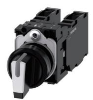
Selector switch, illuminable, 22 mm, round, plastic, white, selector switch, short, 3 switch positions I-O-II, latching, 10:30h/12h/13:30h, with holder, 2x1NO+1NC, screw terminal
