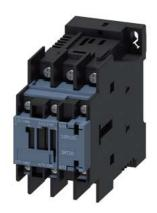
power contactor, AC-3 17 A, 7.5 kW / 400 V 1 NO + 1 NC, 24 V DC with integrated varistor 3-pole, size S0, ring cable lug connection suitable for PLC outputs not expandable with auxiliary switch
