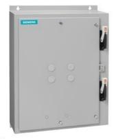
Duplex starter w/o alternator Size 3 Three phase full voltage Solid-state overload relay OLR amp range 25-100A 208VAC 60Hz Coil Combination type Two 100A disconnect switches Encl NEMA type 4 painted steel Water/dust tight weather proof
