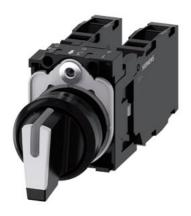
Selector switch, illuminable, 22 mm, round, plastic, white, selector switch, short, 3 switch positions I-O-II, latching, 10:30h/12h/13:30h, with holder, 2 x 1 NO+1 NC, screw terminal, with laser labeling, upper case and lower case, always upper case at beginning of line
