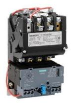
Non-reversing motor starter Size 00 Three phase full voltage Solid-state overload relay OLRelay amp range 3-12A 110-120/220-240VAC 60HZ coil Combination type No enclosure
