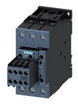
Power contactor, AC-3 65 A, 30 kW / 400 V 2 NO + 2 NC, 84-155 V AC / DC with varistor 3-pole, size S2 screw terminals
