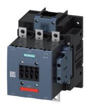
power contactor, AC-3 185 A, 90 kW / 400 V AC (50-60 Hz) / DC operation 110-127 V AC/DC auxiliary contacts 2 NO + 2 NC lateral, permanently mounted 3-pole, frame size S6 busbar connections drive: conventional
