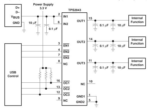
Figure 32. High-Power Bus-Powered Function
