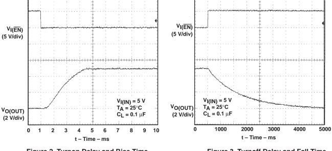
Figure 2. Turnon Delay and Rise Time with 0.1- $\mu\text{F}$  Load
