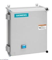
Non-reversing motor starter, Size 2 1/2, Single Phase, 2-Pole, Amb. compensate bimetal OLR, Contactor amp rating 60A, 208VAC 60Hz coil, Non-combination type, Enclosure type 4X fiberglass, Water/dust tight noncorrosive
