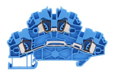
Double-level terminal, Tension-spring connection, Mounting type: Mounting rail TS 35/7.5, Rated cross-section: 2.5 mm², Width: 5.1 mm, Colour: Blue
