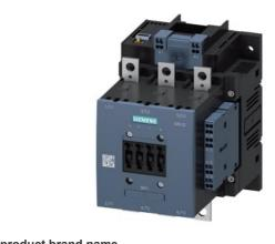
Traction contactor, AC-3 185 A, 90 kW / 400 V Coil 72 V DC x (0.7-1.25) PLC input 24-110 V DC Auxiliary contacts 2 NO + 2 NC 3-pole size S6 Busbar connections Coil connection: Spring-type terminal
