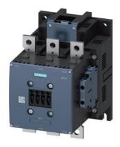
power contactor, AC-3 300 A, 160 kW / 400 V, AC (50-60 Hz) / DC operation 96-127 V AC/DC auxiliary contacts 2 NO + 2 NC 3-pole, frame size S10 busbar connections drive: electronic with PLC interface 24 V DC screw terminal
