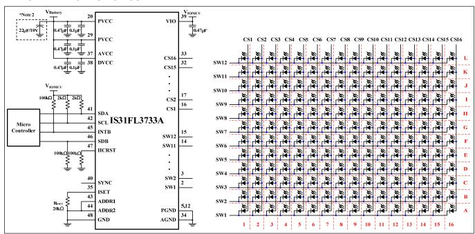
Figure 1 Typical Application Circuit (12×16)
