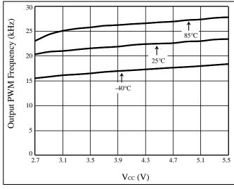
Figure 19 V<sub>CC</sub> vs. CSx PWM Frequency
