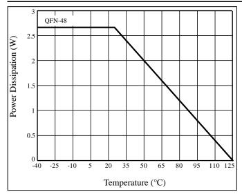
Figure 18 Dissipation Curve
