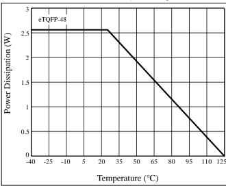
Figure 17 Dissipation Curve
