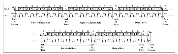
Figure 7 Writing to IS31FL3733A (Automatic Address Increment)
