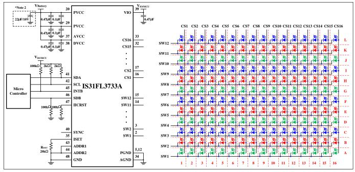
Figure 2 Typical Application Circuit (RGB)
