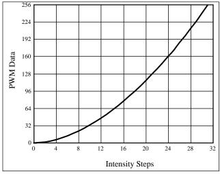
Figure 13 Gamma Correction (32 Steps)
