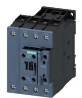
Contactor, AC-1, 60 A/400 V/40  $^\circ\text{C},$  S2, 4-pole, 110 V AC/50 Hz, 1 NO+1 NC, screw terminal
