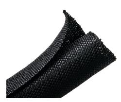
Center-slit overlapping design allows quick and easy access to the wires and cables for future maintenance or inspection without disassembly. Flexible material allows it to easily wrap around a variety of component shapes and sizes, making it easier to use than slit-loom tubing or spiral-wrap materials.
