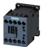
Power contactor, AC-3 7 A, 3 kW / 400 V 1 NC, 24 V DC with diode integrated, 3-pole, Size S00, screw terminal
