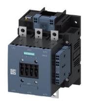
power contactor, AC-3 115 A, 55 kW / 400 V AC (50-60 Hz) / DC operation 21-27 AC/DC, 3 V auxiliary contacts 2 NO + 2 NC 3-pole, frame size S6 busbar connections drive: electronic with PLC interface 24 V DC spring-loaded terminal
