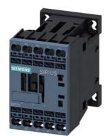
Power contactor, AC-3 12 A, 5.5 kW / 400 V 2 NO + 2 NC 220 V DC, 50 Hz 240 V, 60 Hz 4-pole Size S00 Spring-type terminals
