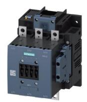
Contactor, AC-1, 275 A/690 V/40 °C, S6, 3-pole, 21-27.3 V AC/DC, PLC-IN optional, with varistor, 2 NO+2 NC, Connection rail/ screw terminal
