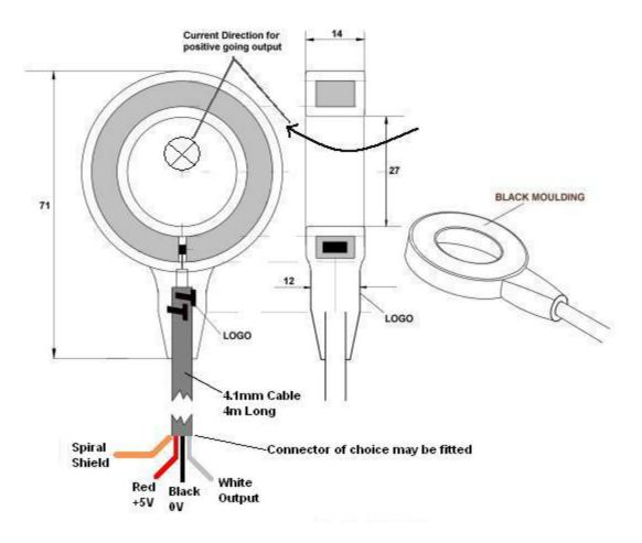
NB: For best accuracy centre primary conductor in aperture
